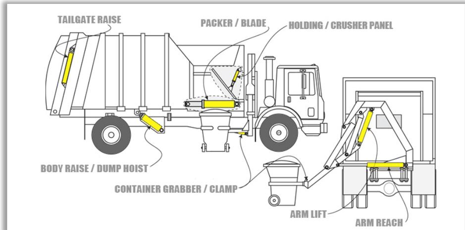
*Figure 3: Side Loader Garbage Truck including Hydraulics Schematic
