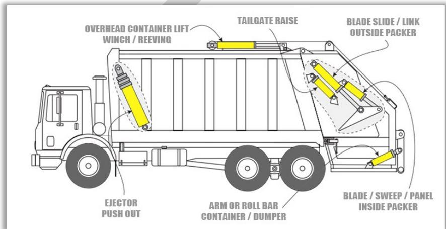
Figure 2: Rear Loading Garbage Truck and Hydraulics Schematic
