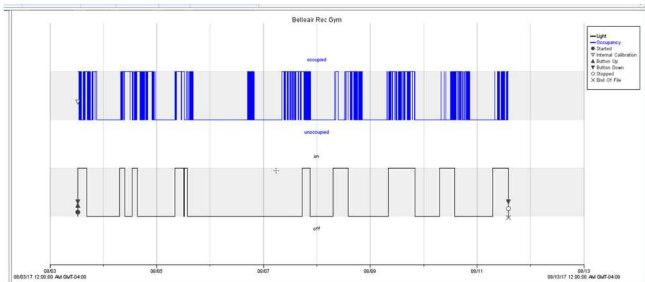
Actual “ON” and “OFF” times can be calculated from this data to determine actual run hours. The graph above shows one full week of data logging. The shaded vertical lines are the different days. As you can see from the graph, the lights for this space typically turn on each based on when people are inside the space. The data from all the loggers is then compiled into an easily referenced format as shown in the following table.
