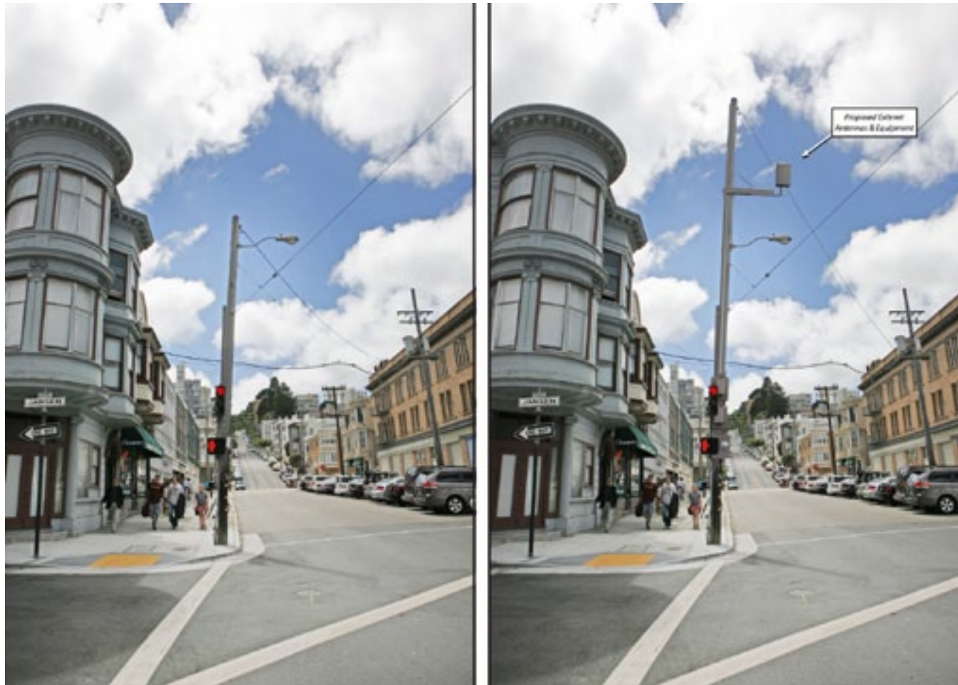
ABOVE: Non-recommended pole height increase (existing pole on left side and previously proposed design on right side) on a signature City-defining street (Lombard Street at Columbus Avenue).
