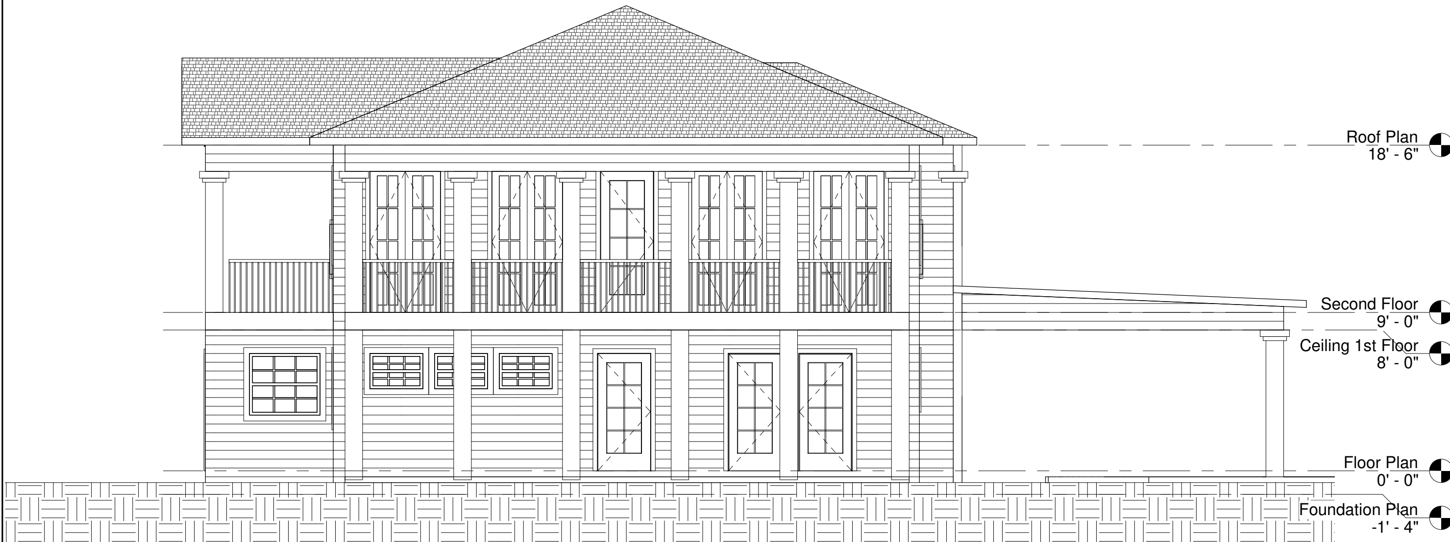
① House East Elevation Existing 3/16" = 1'-0"
