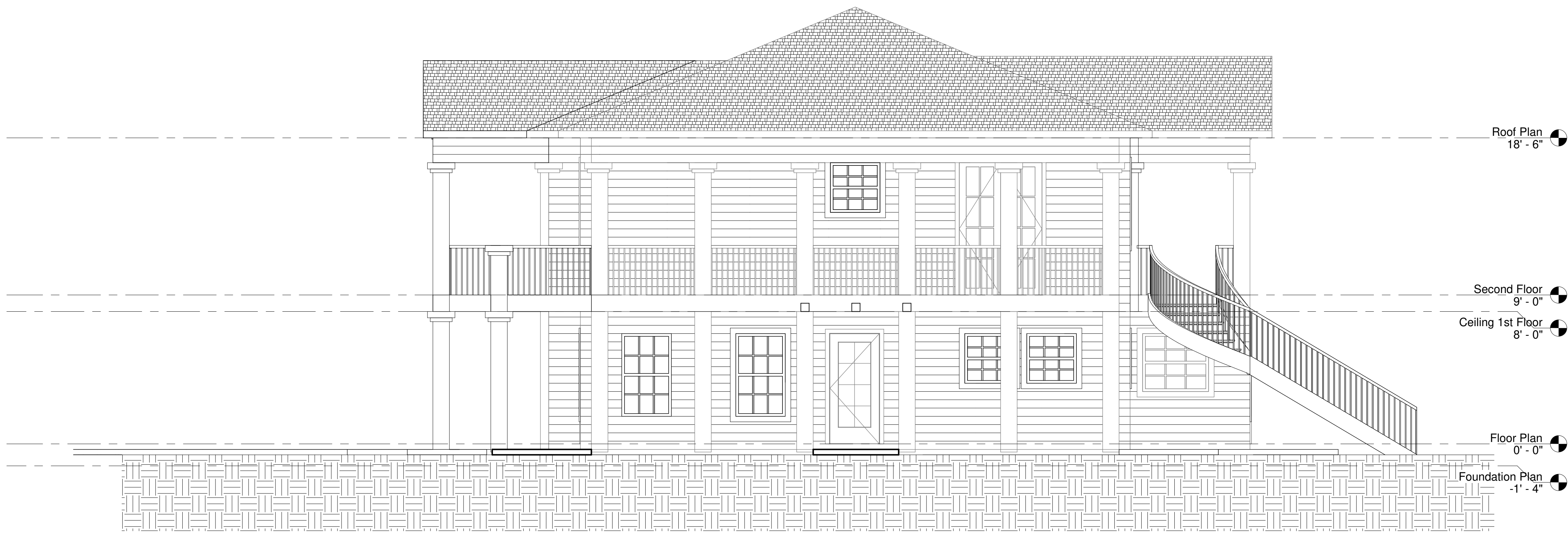
① House West Elevation 1/4" = 1'-0"
