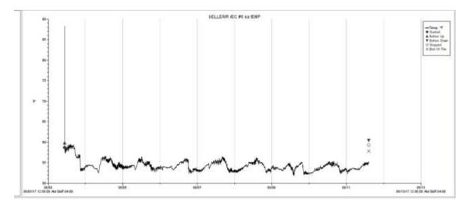
A temperature logger (data taken during the same period as above) shows the supply temperature for an air handling unit (AHU) serving the Dimmitt Community Center gym. Looking at the temperature logger data, it is very easy to ascertain the runtime, supply temperature, and relative humidity for these air handling units. These variables are used in the energy savings calculations to calculate the guaranteed savings for the project.
