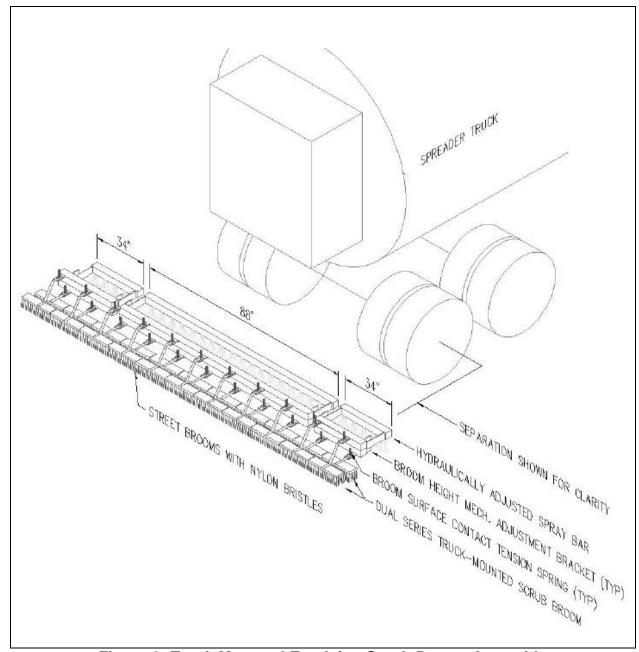
Figure 2: Truck Mounted Emulsion Scrub Broom Assembly
