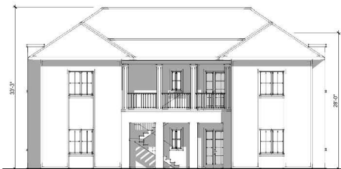
TYPICAL WEST ELEVATION
